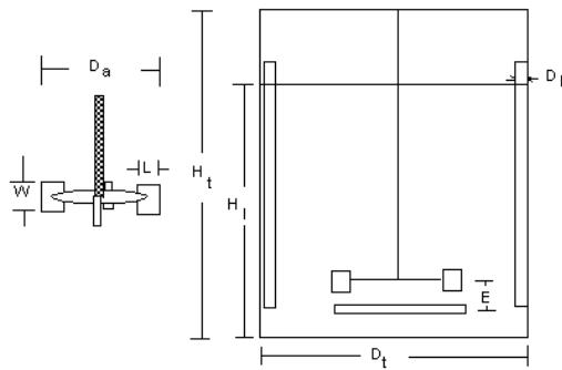
A stirred tank bioreactor is approximately cylindrical in shape. It has a total volume ( $V_t$ ) of 100,000 liters. The geometry of the reactor is defined by the following ratios:  $D_t:H_t=0,5$  ;  $D_a:D_t=0,33$  ;  $D_b:D_t = 0,1$
