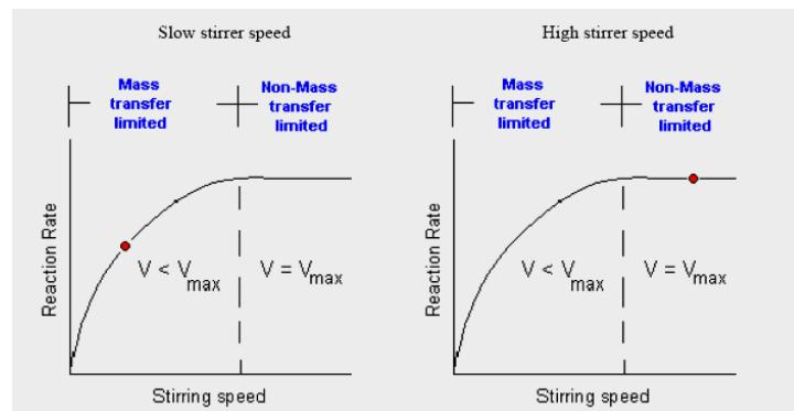
Figure 1: If the bulk liquid is well mixed, the convective transport of oxygen through the bulk liquid is much faster than compared to the diffusion in the liquid films.
